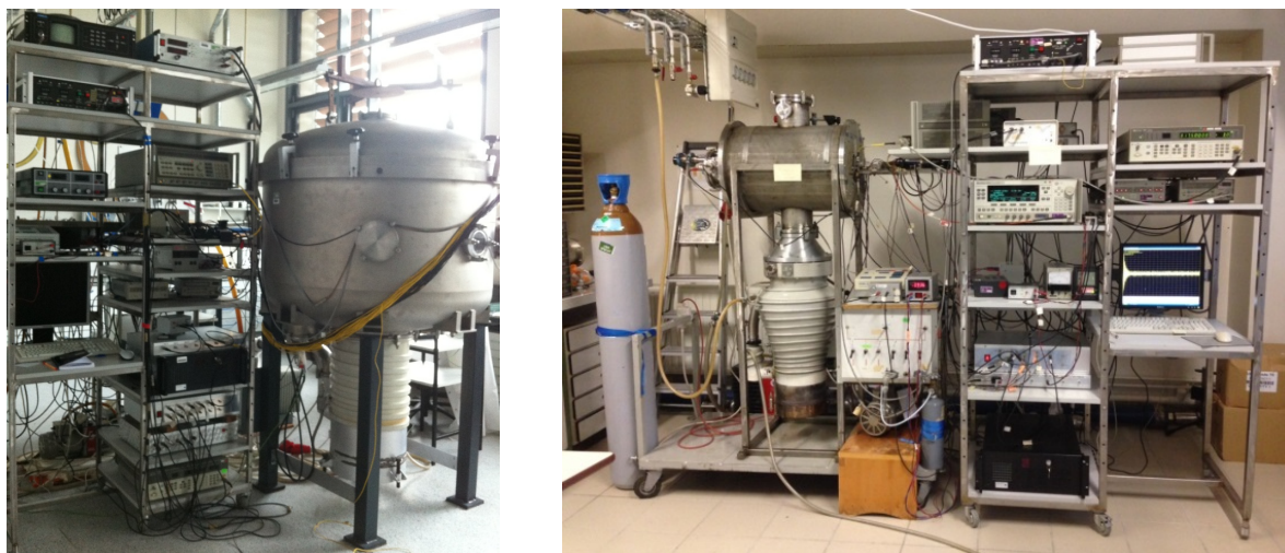
FIG. 2. MJ-FTMW spectrometers used in this work, located in Aachen (2-26.5 GHz) and in Paris (26.5-40.0 GHz).
