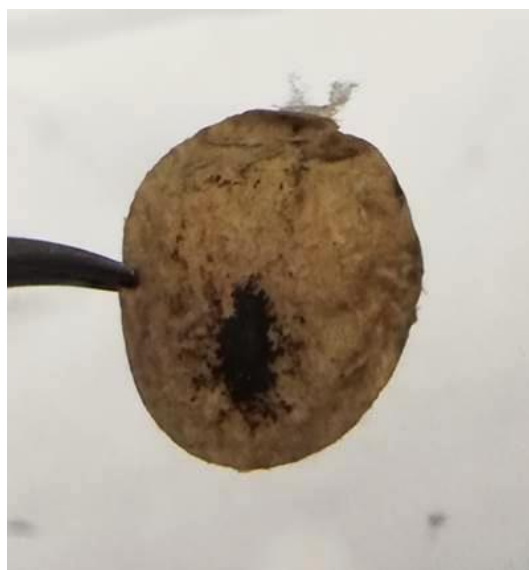
Figure 93: Separator recovered from the cycled Ca/S cell. The yellow color is indicator of polysulfide dissolution and diffusion in the electrolyte during cycling. 205
