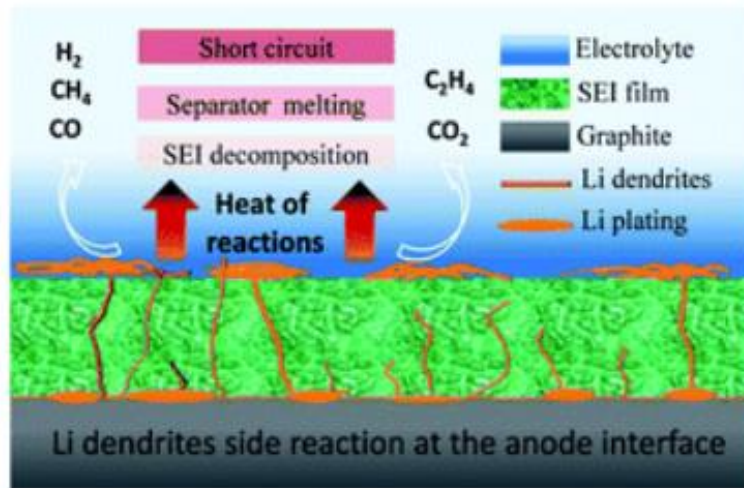
Figure 18: Scheme of phenomena responsible for LIBs failure. 35
