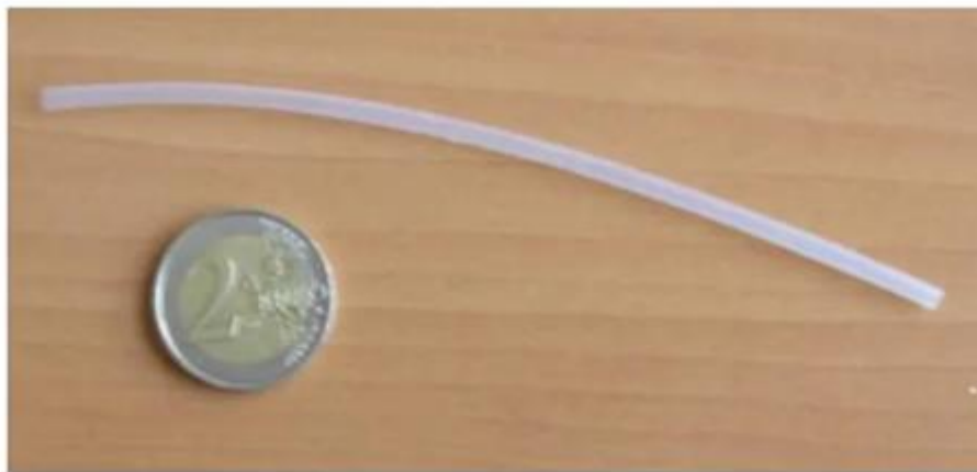
Figure 675. Extruded tube of plasticized P(VDF-TrFE-CTFE).
