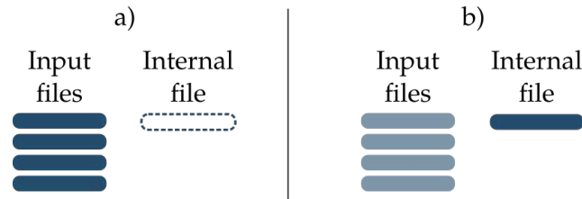
Figure 2.5: a) In the case where no internal file already exists, the input files are considered as the default Knowledge Base of the agent b) In the case where an internal file exists for a given agent, this means that the robot is already interacting with this agent. In the latter case, the input files are not taken into account and the previously estimated Knowledge Base of the agent is loaded. If the current Knowledge Base represents that the robot’s one, the robot simply restarts with its previous knowledge base.
