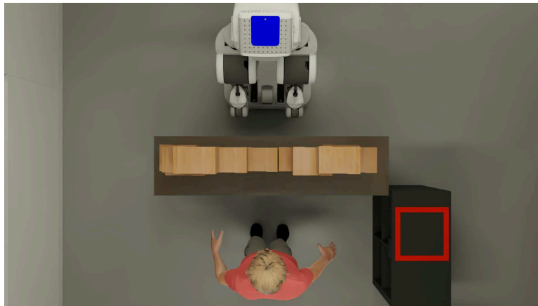
Figure 9.3: The Director Task setup with the robot and the human partner one in front of the other and a piece of furniture between them. Compartments are placed on top of the furniture and blocks are placed in the compartments. Next to the agent having the receiver role, here the human, a storage area is placed to drop the removed blocks.
