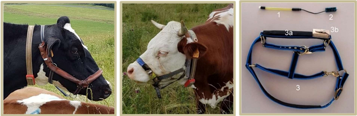
Figure I.6. Head collars containing MSR pressure sensors: a flexible tube containing oil (1) is linked to a MSR 145 electronic sensor (2) and inserted in the noseband (3a = oil tube, 3b = sensor) of a regular head collar (3). (Photos S. Zurmühle 2017 and Braun et al. 2013).
