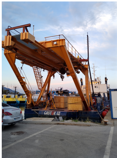
Figure 2.10: Boat from the Foselev Marine company used to transport the DUs during the sea operation and deploy them.
