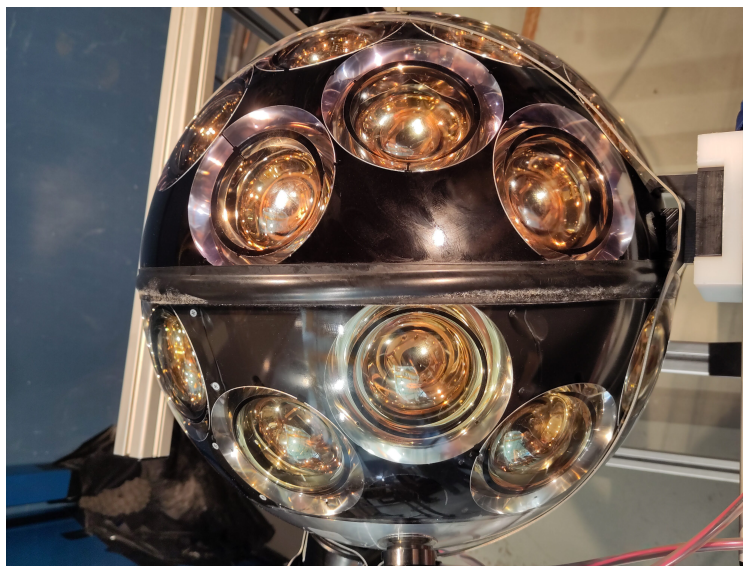
Figure 2.2: Design of the DOM with the PMTs at its surface.
