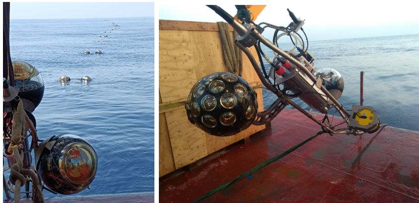
Figure 2.6: A storey with the OMs from ANTARES during the dismantling is shown on the left. More storeys can be seen stretching to the horizon in the water. On the right side a KM3NeT DOM incorporated to an ANTARES DU for testing the multi-PMTs technical design.
