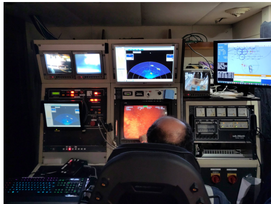
Figure 2.13: The pilots of the ROV with the camera, sonar and boat position.
