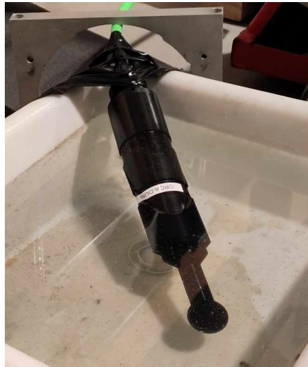
Figure 2.36: A KM3NeT hydrophone connected to BM during an acoustic calibration test at CPPM.
