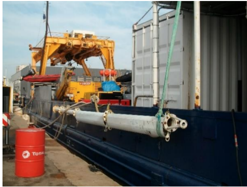
Figure 2.25: Mechanical arm with the transducer on the Castor boat.
