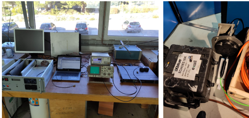
Figure 4.3: Installation and cabling of the emission system at CPPM.
