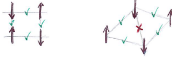
Figure 1.5: Geometrical frustration on lattice spin systems. Considering the Ising model with anti-ferromagnetic interactions favoring links between \uparrow and \downarrow spins, the square lattice favors all bonds in the ground state, while the triangular lattice does not. Indeed, as shown on the right sketch, for all the links with green ticks to be satisfied, there has to be an unsatisfied one, marked with a red cross.
