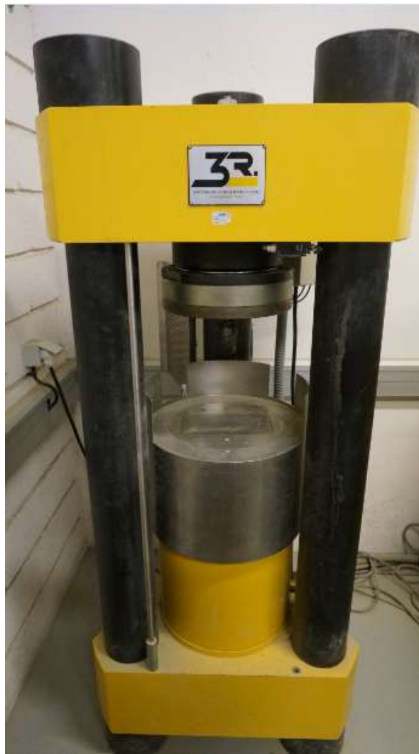
Figure 3.9. 3R 3000 TC/TH compression press.
