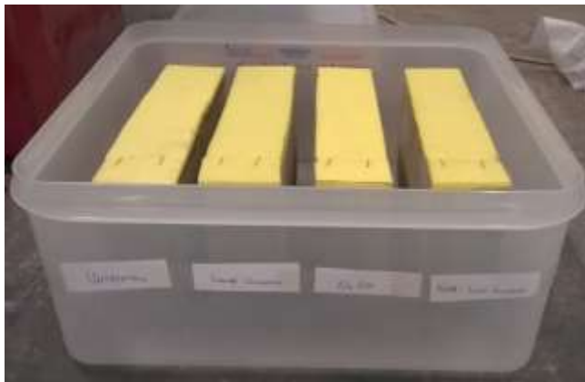
Figure 7.3. Set- up of contact test
