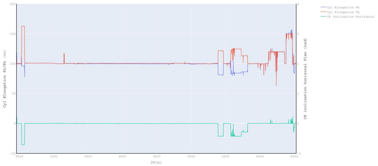
A.2. 9 Evaluation of the cutter head inclination (horizontal plane) vs TBM chainage. The inclination is calculated by using elongation of cylinders located at 4h and 8h. Right axis shows cylinder's elongation in mm. Left axis demonstrates inclination fluctuation of cutter head during each meter of advancement.
