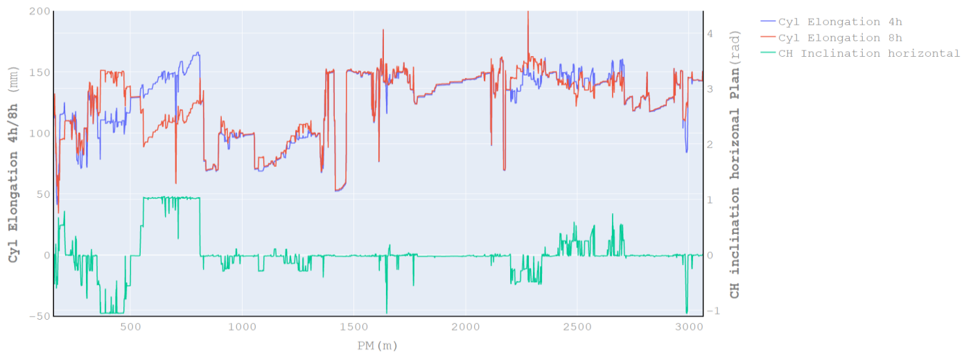
Figure 3-23 The cutter head inclination evolution and elongation of displacement cylinders 4h-8h
