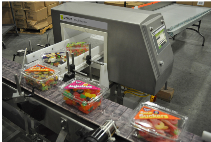
Figure 1.2.3: Metal detection system integrated into the production line in the food industry [23].
