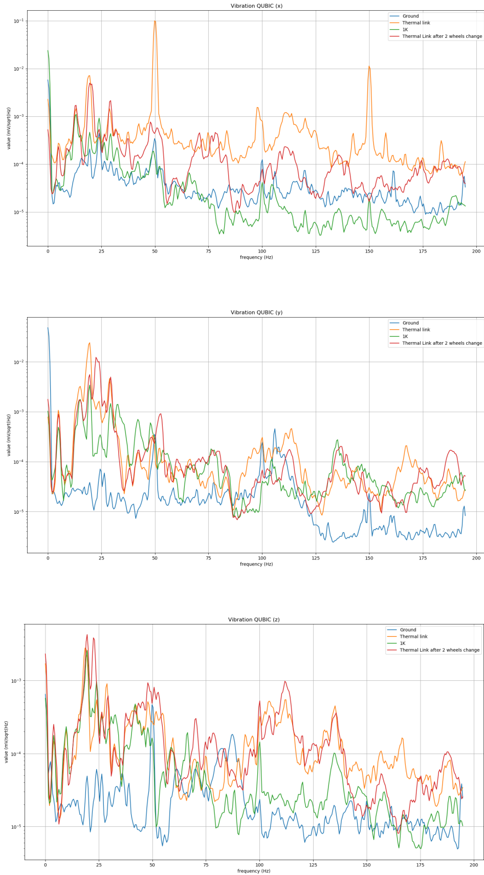
Figure 4.21: Top : vibrations of the 300 mK link on X, Y and Z axis from top to bottom.
