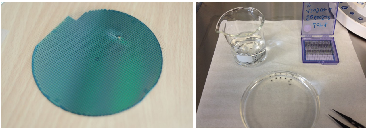
Figure 4.30: Left : A full wafer sent by StarCryo, all the SQUID are lightly stick together. Right : Cleaning set at the APC cleaning room. Credit : Damien Prêle
