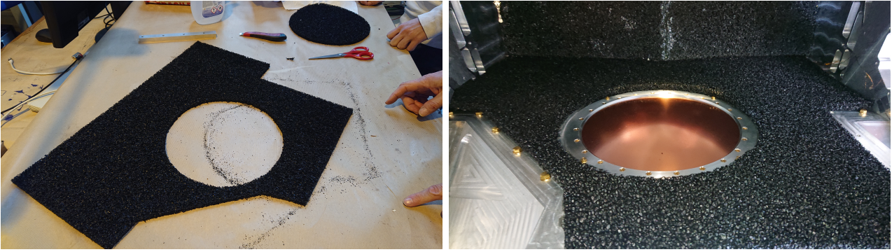
Figure 4.38: Installation of the Eccosorb HR-10 on the inside of the 1 K box.
