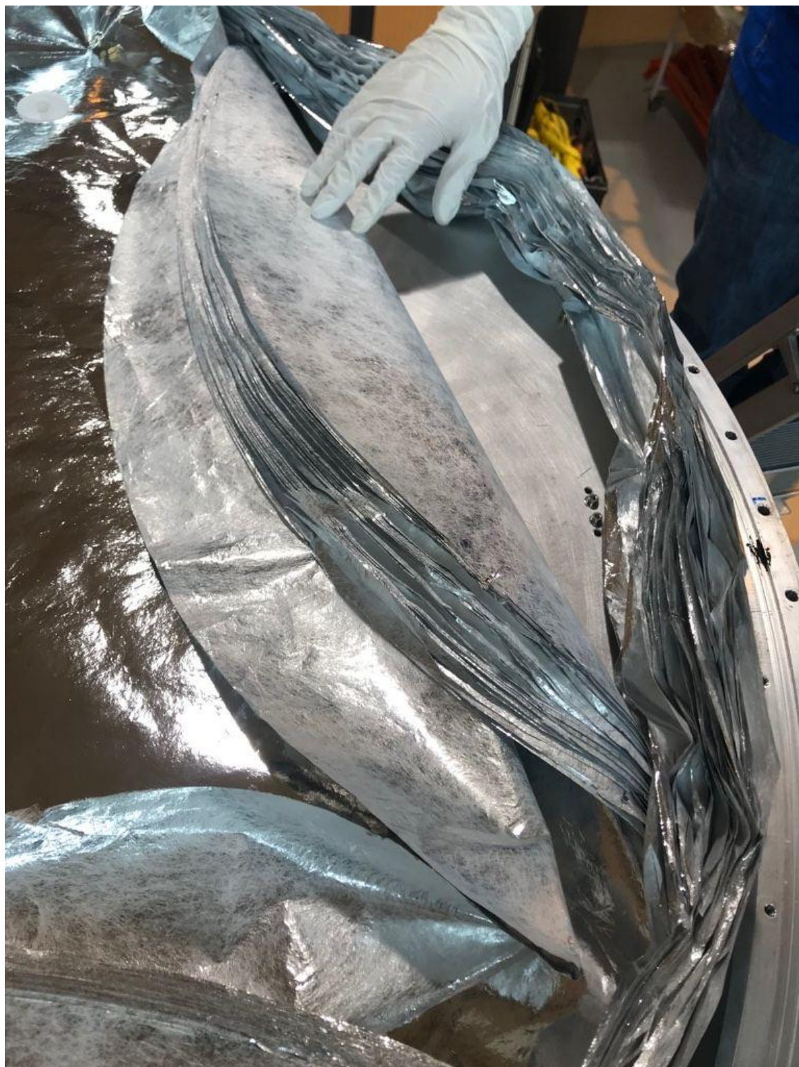
Figure 4.13: MLI layers on the 40 K top cover. There is 30 layers on the flange and 30 layers on the cover in order not to break the cryogenic continuity of the layers.
