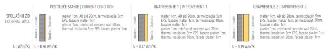
Figure 37. Energy performance improvement for external wall of residential buildings for multi-family houses in BIH made at the end of XX and beginning of the XXI century (Arnautovic-Aksic et al. 2016)
