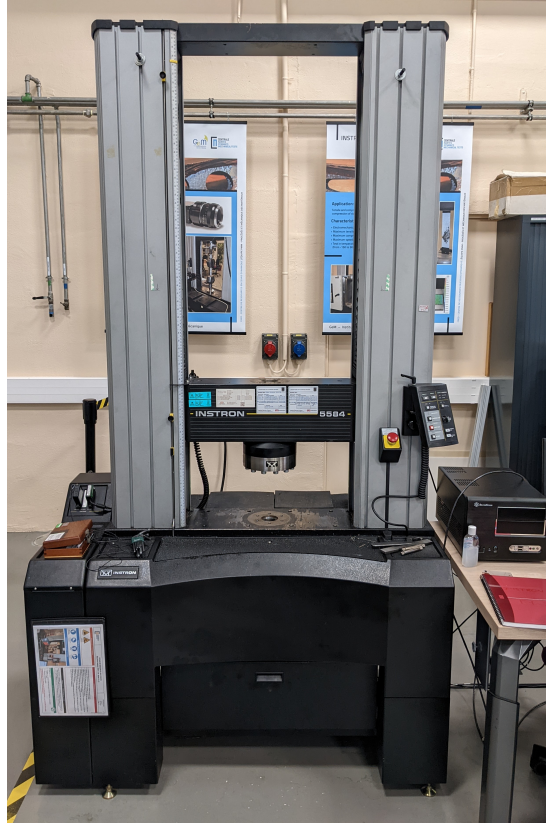
Figure 6.6: Instron 5584 used for testing.
