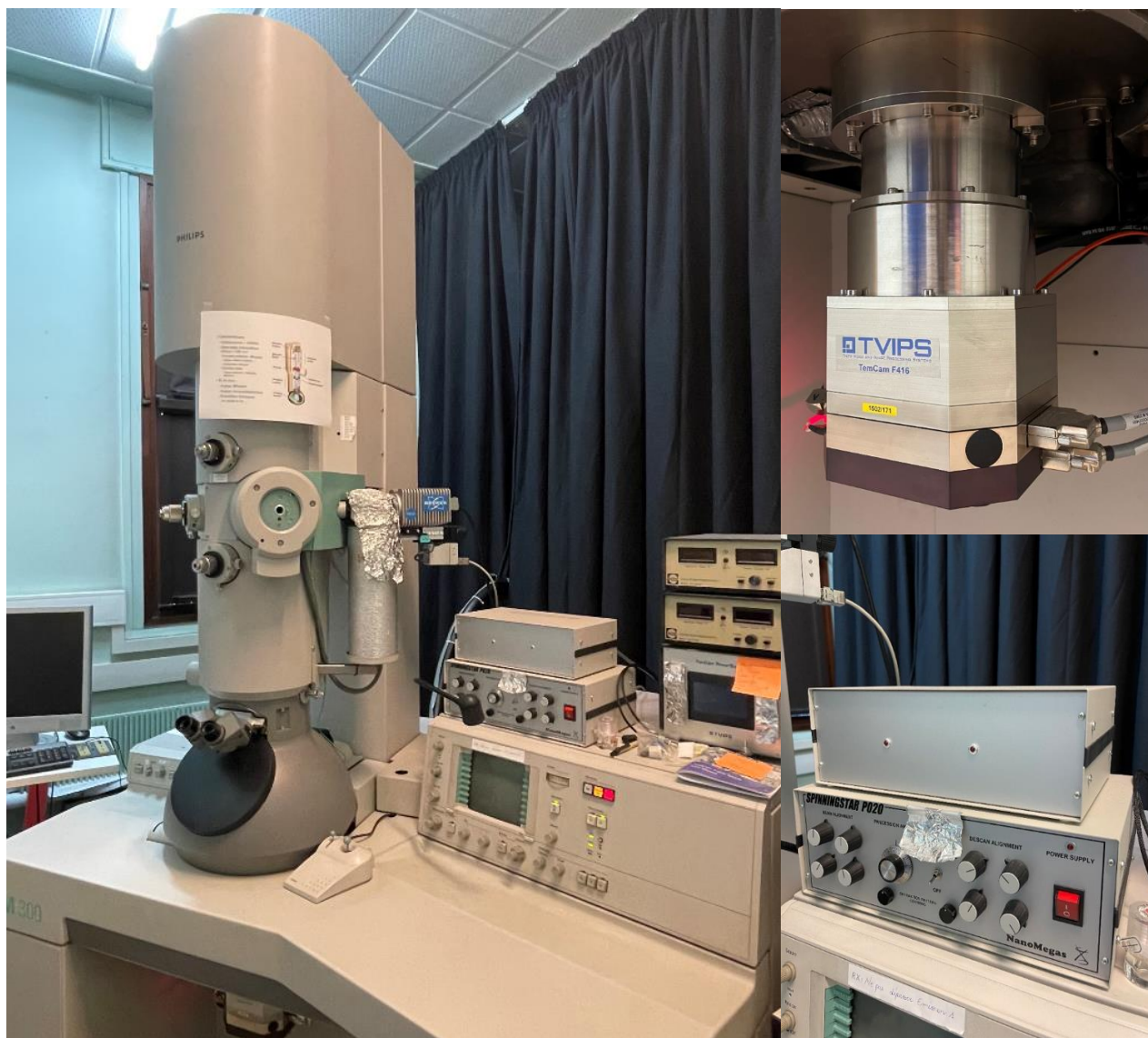
Figure 2.11: The Philips CM300 ST TEM used throughout this thesis is shown on the left. The TVIPS F416 CMOS camera used for recording diffraction patterns and images is shown on top right, and the Nanomegas Spinning star device used to generate a precessed beam is shown in bottom right.
