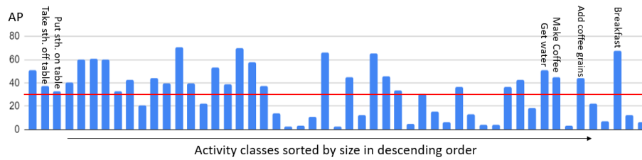
Figure 6.3: Average Precision for the actions in TSU. The classes are sorted by their size. The mAP is marked by a red line. We can see that while there is a slight trend for smaller classes to have lower accuracy, many classes do not follow that trend.
