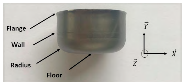
Figure 3.6 – Definition of the cup coordinate system used for the measurements
