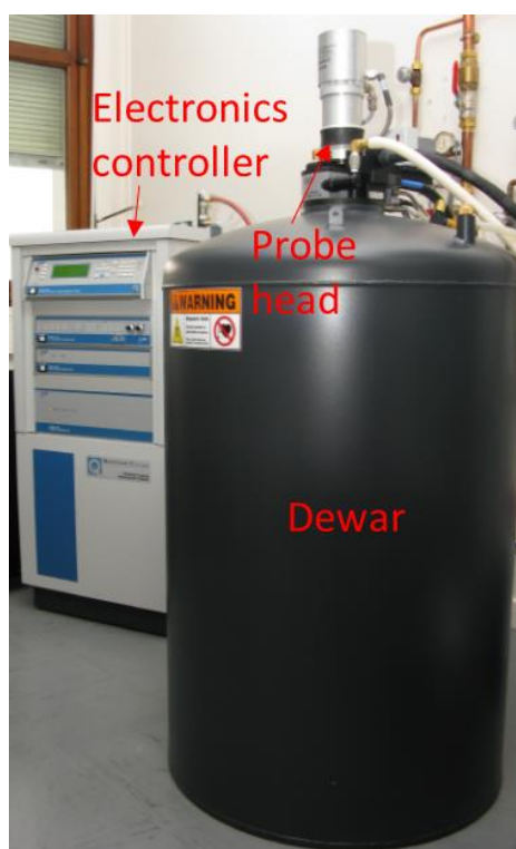
Figure 3.22 PPMS set-up at Néel Institute (Grenoble).
