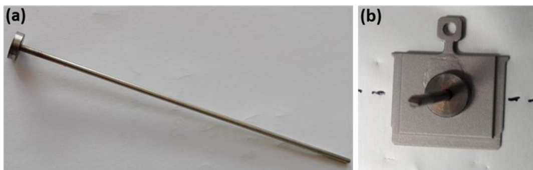
Figure 4.1 (a) Stainless steel rod (pin) having a disk shape terminated side and (b) the plate- \text{Cr}_2\text{AlC} -pin system after mild annealing at 80^\circ\text{C} .
