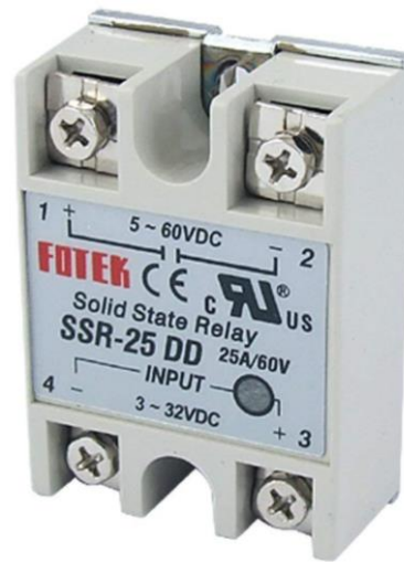
Figure 5.4: Solid state relay SSR-25 DD. Standard type DC to DC. The input voltage ranges between 4 and 32 Volts. The response time is estimated to 1 ms [121].
