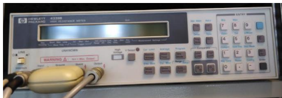
Figure II. 11: The Hewlett Packard 4339B High Strength Resistivity Meter used at LPCA
