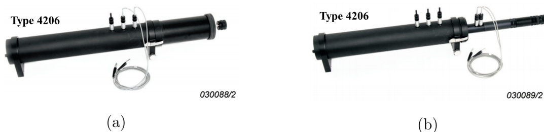
Figure 7.3: Setup images of (a) Kundt's large tube of 100 mm diameter, (b) small tube of 29 mm diameter [3].
