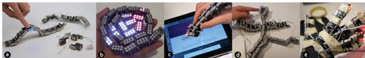
Figure 1.8: Device and application examples of the ChainFORM hardware system. a: ChainFORM hardware configurations and modules, b: reconfigurable display, c: shape changing stylus, d: animated character, e: haptic glove [189].
