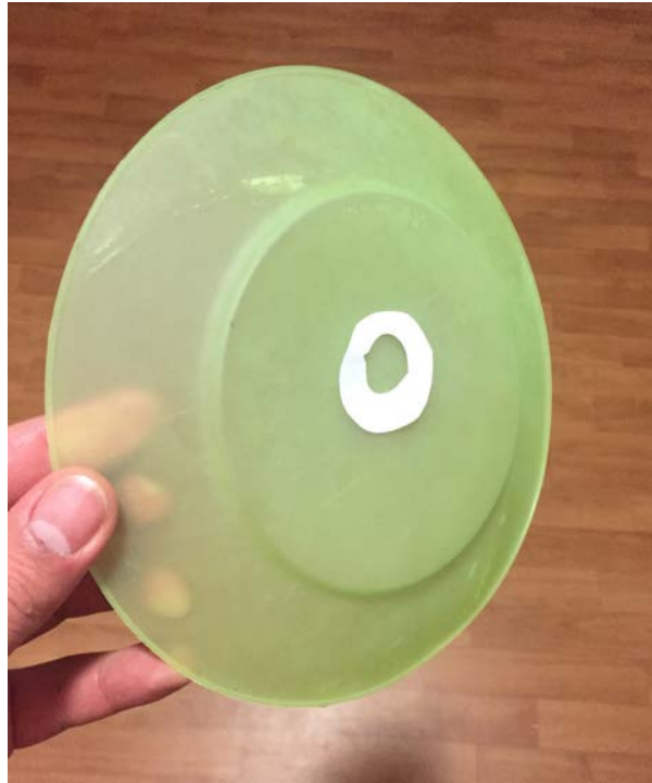
Figure 6.3: A food plate used in this application equipped with a RFID tag.
