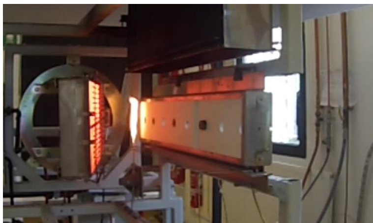
Figure 4-3 : Calibration du flux incident
