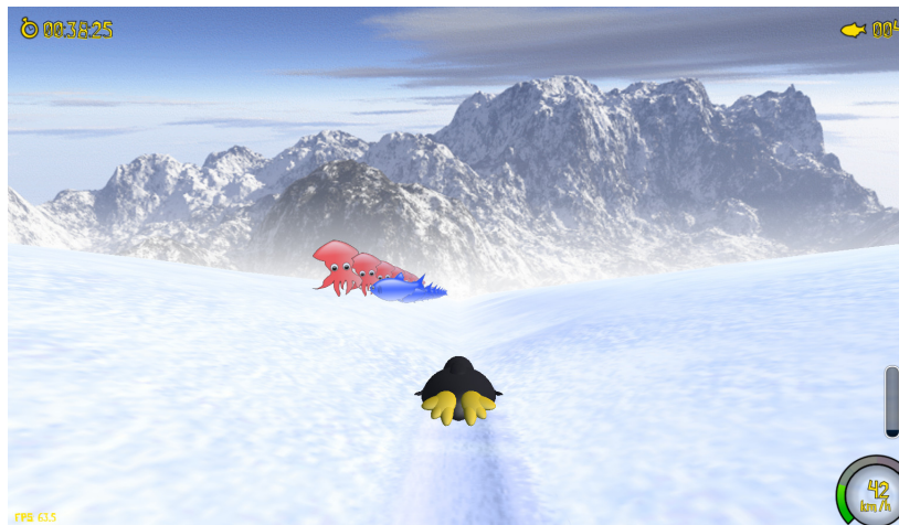
Figure 4.4: Screen-shot of the Tux Racer game, customized for synchronous MI BCI. Here, the penguin already passed the flag denoting the beginning of the trial. An additional row of reward (squid) was added to reduce frustration, and increase motivation.
