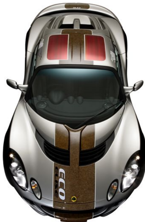
Fig. 1. The Lotus Eco Elise is manufactured using sustainable hemp technical fabrics as the primary constituent in the composite body panels and spoiler. Car dimensions are 3726 mm × 1719 mm × 1202 mm [15].
