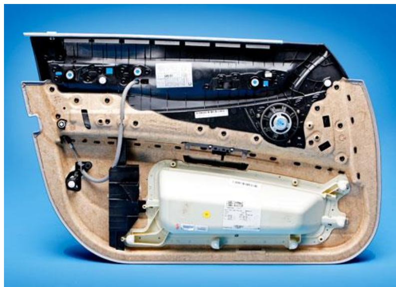
Fig. 2. Automotive door panel made with flax fibres [21]. Dimensions of about 1 m.
