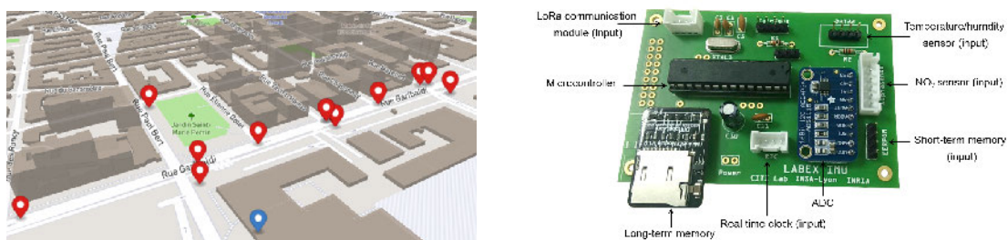
Figure 3.5: Deployment case study of the UrPolSens platform. From left to right: (a) the map of the 12 sensors (red) and the gateway (blue) that we deployed in the downtown of the Lyon city; and (b) a zoom on the main circuit of our sensor nodes.
