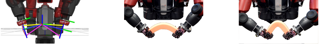
FIG. 5.5 Bend at the centre: The absolute pose was fixed at the centre of the foam. The initial desired state of VSs is shown in yellow, current desired state in blue, and final desired configuration in magenta.
