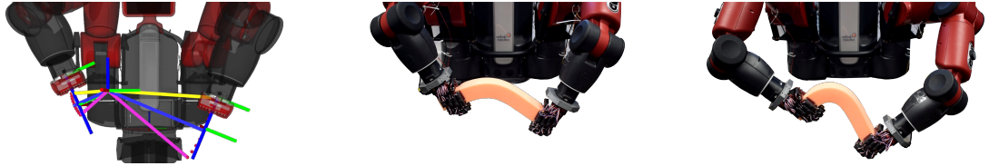
FIG. 5.6 Bend off centre: The absolute pose was shifted 10 cm to the left from the centre of foam.
