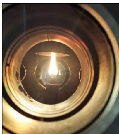
Figure 3.1. Laser pyrolysis flame of ethylene, argon and nitrates precursors without air
