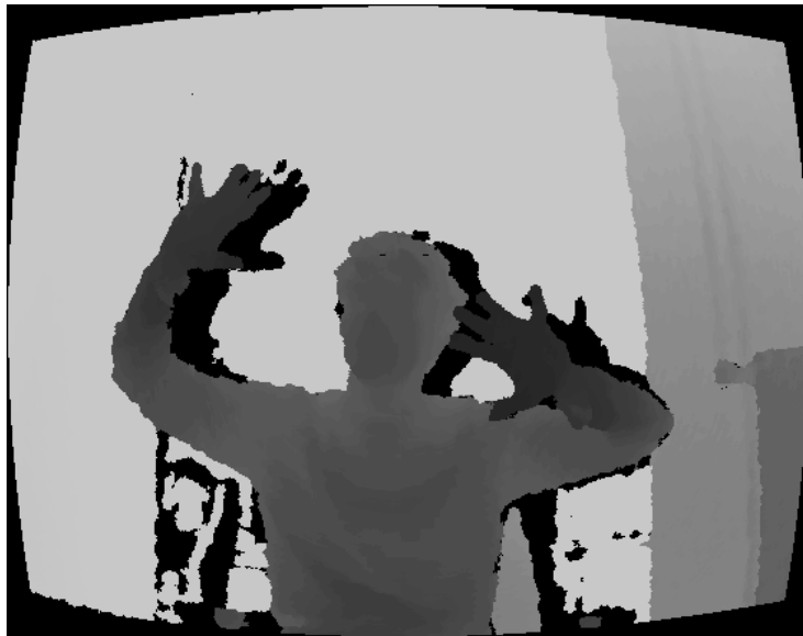
Figure 3.6: Example of Kinect range image. In this case, the range image is the direct output of the Kinect sensor, thus no additional projection is required. Courtesy of Vincent Weistroffer, Robotics Laboratory (CAOR), MINES ParisTech, 2012.
