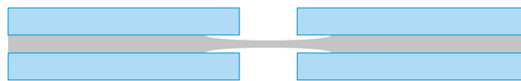
Figure 11 How the interlayer is stretched and debonded from the glass under impact
