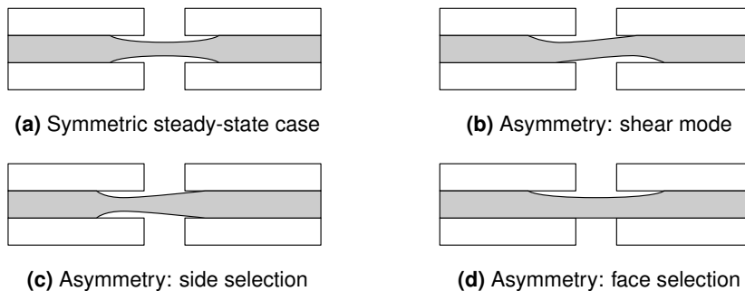
Figure III.7 Interfacial delamination behaviors: scenarii of divergence from steady state at low adhesion
