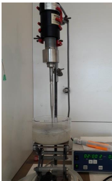
Fig. 2.2. Photo of the ultrasound equipment (HD 2070, Bandelin, Germany) used to disperse nanoclay in the casting dispersion.
