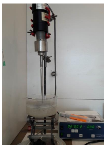
Fig. 3.1. Photo images of the ultrasound equipment used to disperse nanoclay in the casting dispersion (reproduced from chapter 2).
