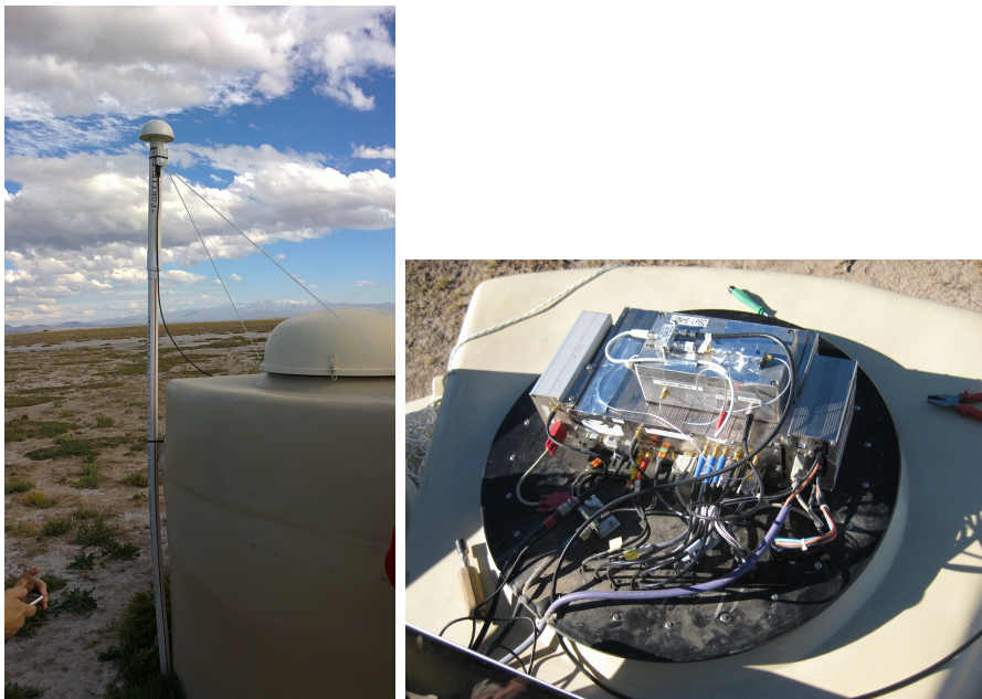
Figure 4.8: Left: antenna integrated with the SD tanks. Right: EASIER electronics box on top of the SD electronics.
