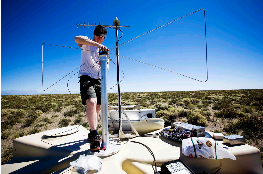
Figure 3.20: Left: Butterfly antennas installed on a water Cherenkov tank. Right: picture of the two electronic boxes.
